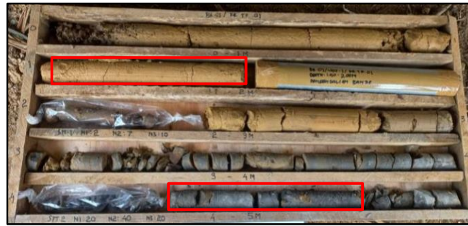
Figure 5. Claystone samples at drill point BH-01 at a depth 4-15 meter
