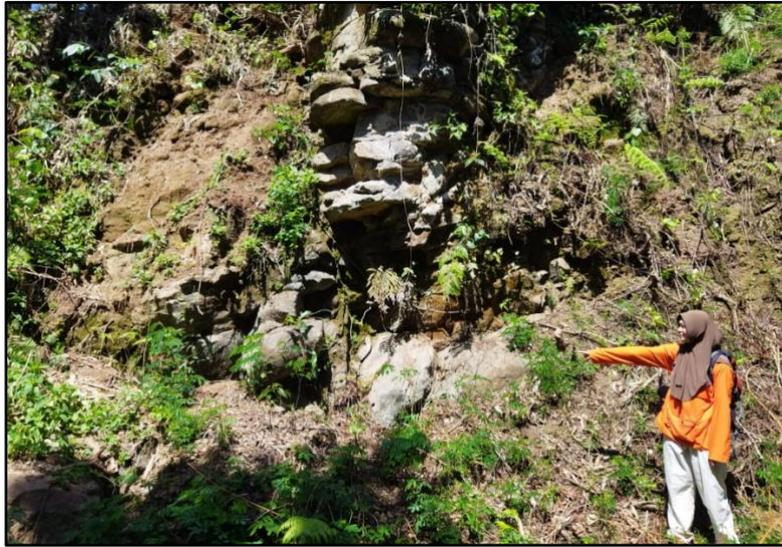
Figure 1 Appearance of station 1 represents the degree of weathering IV with a photographic direction N 215° E
