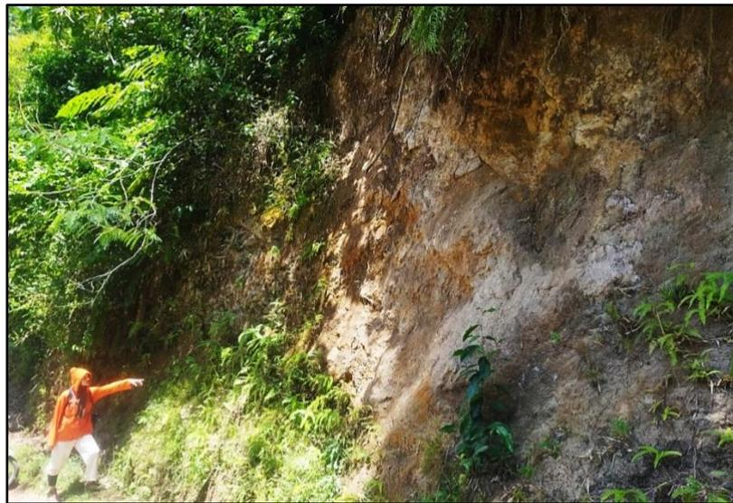
Figure 2 The appearance of station 3 represents the degree of weathering V with the photo direction N 141° E caused by biological weathering and chemical weathering
