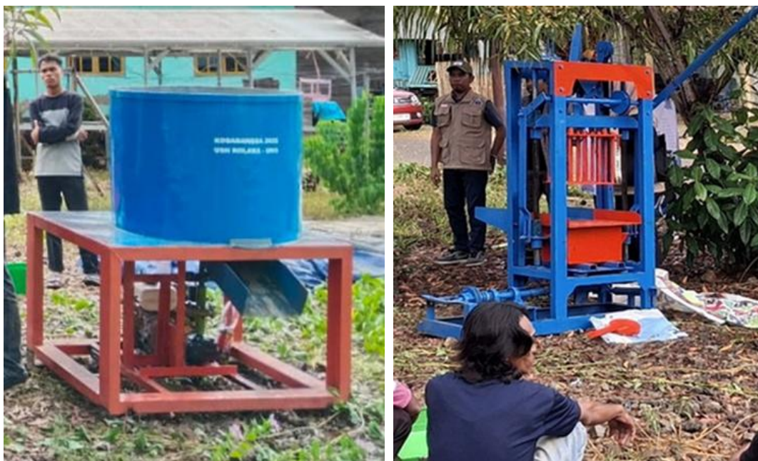
Figure 1. Mixer and Brick Press Machines for Kosabangsa 2025 Program in Tambea Village
